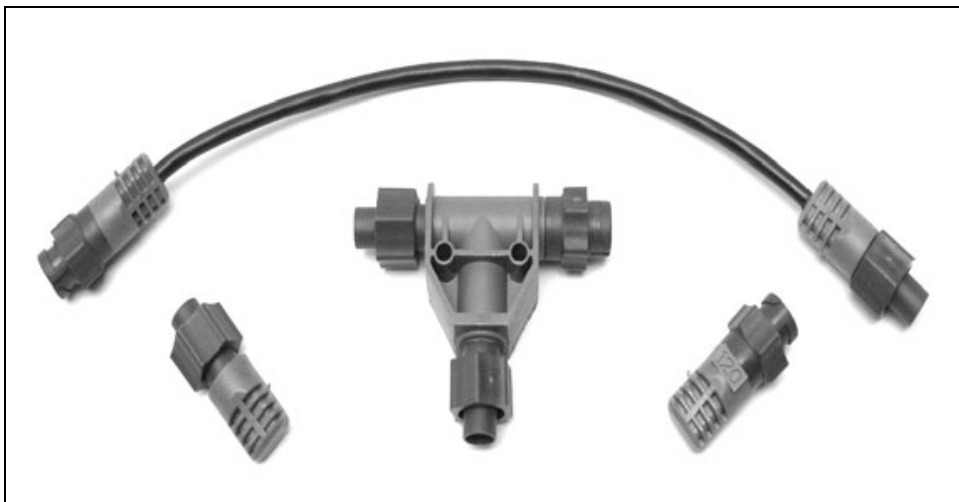
LowranceNET Node Kit for a NMEA 2000 network. Includes a 2 foot extension cable, T connector, 120-ohm male terminator and 120-ohm female terminator.
